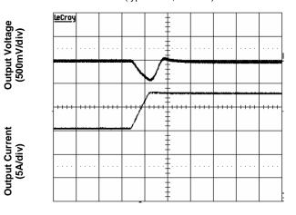
Time - t (200µs/div) Figure 6. Transient Load Response (typical Vin, load current steps from 50% to 75% at a slew rate 0.1A/µs)
