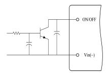
Figure 10. Open Collector Enable Circuit
