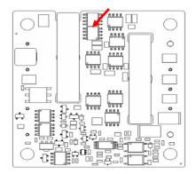
Figure 14. Temperature Monitoring Location
