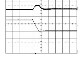
Time - t (200µs/div) Figure 5. Transient Load Response (typical Vin, load current steps from 75% to 50% at a slew rate 0.1A/µs)
