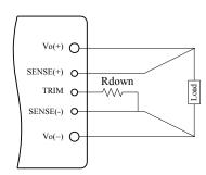
Figure 12. Circuit to Decrease Output Voltage
