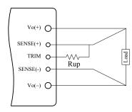
Figure 13. Circuit to Increase Output Voltage
