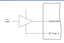
Figure 11. Direct Logic Drive
