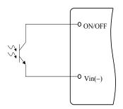
Figure 9. Opto Coupler Enable Circuit
