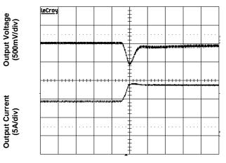
Time - t (100µs/div) Figure 6. Transient Load Response (typical Vin, load current steps from 50% to 75% at a slew rate 0.1A/µs)
