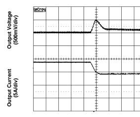
Time - t (100µs/div) Figure 5. Transient Load Response (typical Vin, load current steps from 75% to 50% at a slew rate 0.1A/µs)
