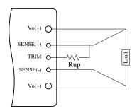
Figure 14. Circuit to Increase Output Voltage
