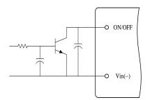
Figure 11. Open Collector Enable Circuit
