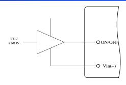
Figure 12. Direct Logic Drive
