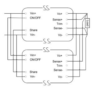
Figure 15. Circuit Configuration for Active Current Share
