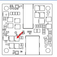
Figure 16. Temperature Monitoring Location
