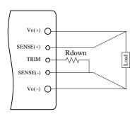
Figure 13. Circuit to Decrease Output Voltage
