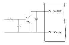
Figure 11. Open Collector Enable Circuit
