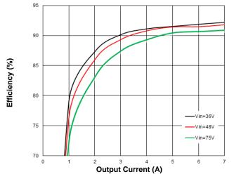
Figure 1. Efficiency vs. Load Current (25°C)
