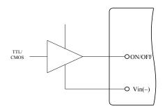
Figure 12. Direct Logic Drive
