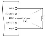
Figure 14. Circuit to Increase Output Voltage
