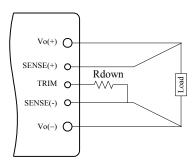
Figure 13. Circuit to Decrease Output Voltage
