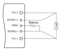
Figure 17. Circuit to Decrease Output Voltage
