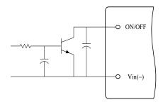
Figure 15. Open Collector Enable Circuit
