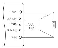
Figure 18. Circuit to Increase Output Voltage
