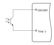
Figure 14. Opto Coupler Enable Circuit
