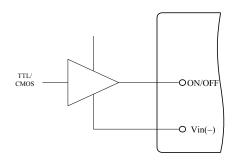
Figure 16. Direct Logic Drive
