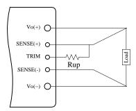
Figure 13. Circuit to Increase Output Voltage
