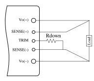
Figure 12. Circuit to Decrease Output Voltage
