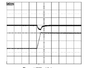
Time - t (200µs/div) Figure 6. Transient Load Response (typical Vin, load current steps from 50% to 75% at a slew rate  $0.1A/\mu s$ )
