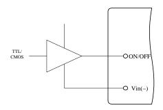
Figure 11. Direct Logic Drive
