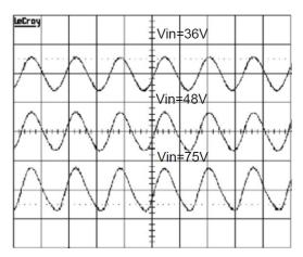
Time - t (2µs/div) Figure 3. Output Ripple Voltage at Full Load
