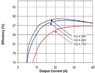
Figure 1. Efficiency vs. Load Current (25°C)
