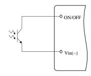
Figure 9. Opto Coupler Enable Circuit
