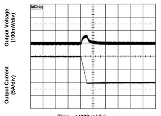
Time - t (200µs/div) Figure 5. Transient Load Response (typical Vin, load current steps from 50% to 25% at a slew rate  $0.1A/\mu s$ )
