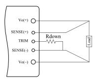
Figure 13. Circuit to Decrease Output Voltage
