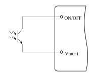
Figure 10. Opto Coupler Enable Circuit
