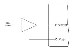
Figure 12. Direct Logic Drive
