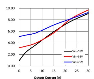
Figure 2. Power Loss vs. Load Current (25°C)
