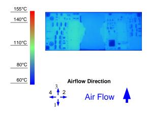
Figure 8. Thermal Image for Airflow Direction 3 (30A output, 55°C ambient, 200 LFM, typical Vin, open frame, socket interface)
