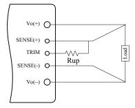
Figure 14. Circuit to Increase Output Voltage
