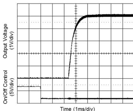
**Figure 7** Output voltage monotonic startup
