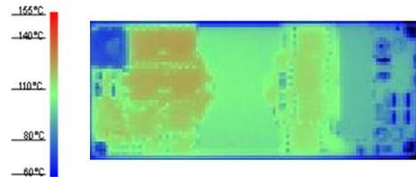
**Figure 10** Thermal image of a power module
