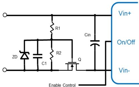
**Figure 3** Typical Inrush Current Control Circuit
