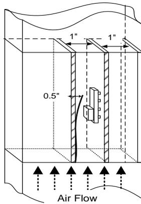
**Figure 8** Wind-tunnel setup
