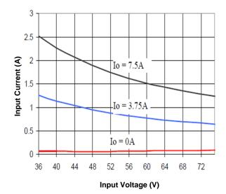
Figure 2. Input Characteristics
