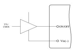
Figure 12. Direct Logic Drive
