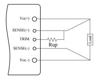
Figure 14. Circuit to Increase Output Voltage
