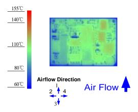
Figure 8. Thermal Image for Airflow Direction 1 (4.2A output, 70°C ambient, 0LFM, typical Vin, open frame, unit soldered onto a fixture board.)
