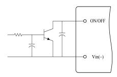
Figure 11. Open Collector Enable Circuit
