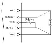
Figure 13. Circuit to Decrease Output Voltage
