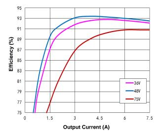
Figure 1. Efficiency vs. Load Current (25°C)
