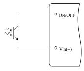
Figure 10. Opto Coupler Enable Circuit
