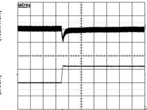
Time – t (500μs/div) Figure 8. Transient Load Response (typical Vin, load current steps from 50% to 75% at a slew rate 0.1A/μs)
