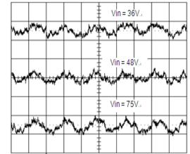
Time - t (2µs/div) Figure 4. Input Reflected Ripple Current at Full Load
