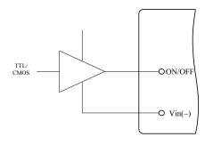
Figure 14. Direct Logic Drive
