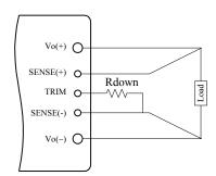
Figure 15. Circuit to Decrease Output Voltage
