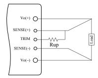
Figure 16.Circuit to Increase Output Voltage
