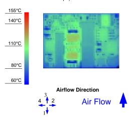
Figure 10. Thermal Image for Airflow Direction 3 (25A output, 55°C ambient, 0 LFM, typical Vin, open frame, unit soldered onto a fixture board)
