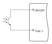
Figure 12. Opto Coupler Enable Circuit
