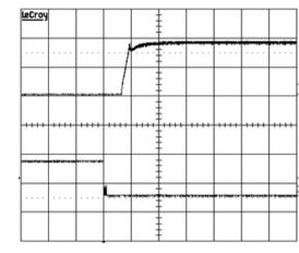
Time - t (5ms/div) Figure 6. Start-Up from Enable Control (typical Vin, full load)
