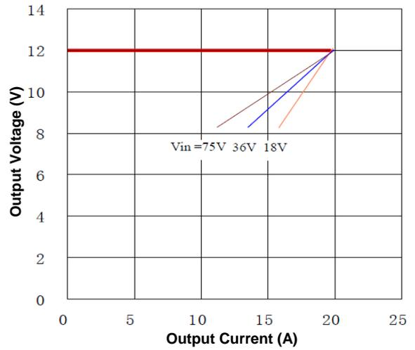
Figure 10. Output Characteristics
