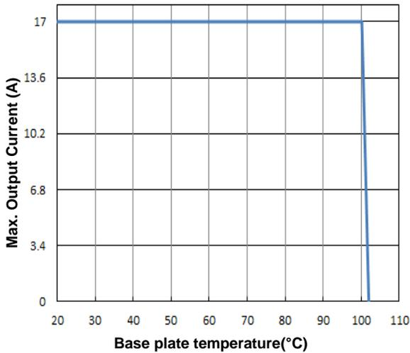
Figure 13. Current Derating Curve for Base plate
