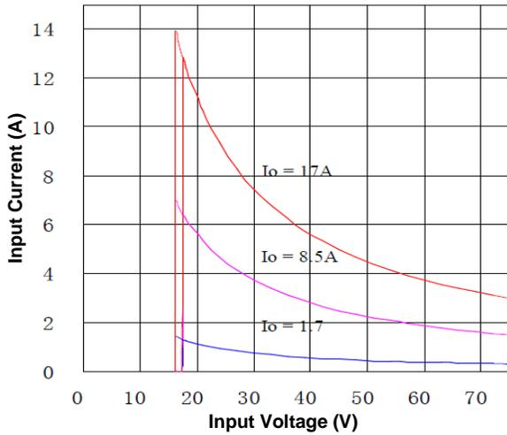
Figure 9. Input Characteristics
