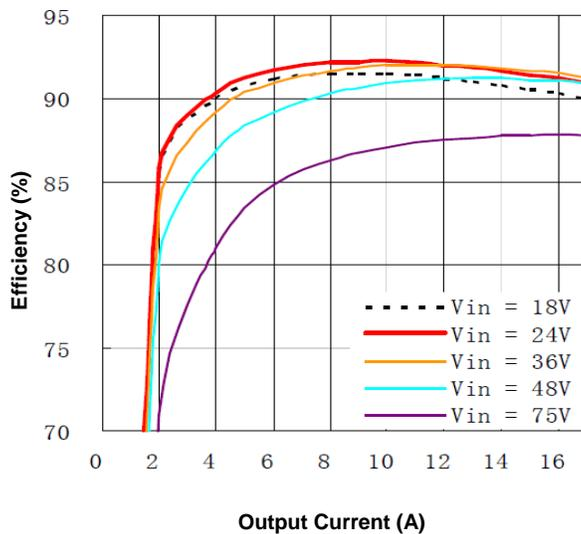
Figure 1. Efficiency vs. Load Current
