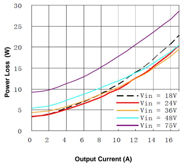
Figure 2. Power Loss vs. Load Current
