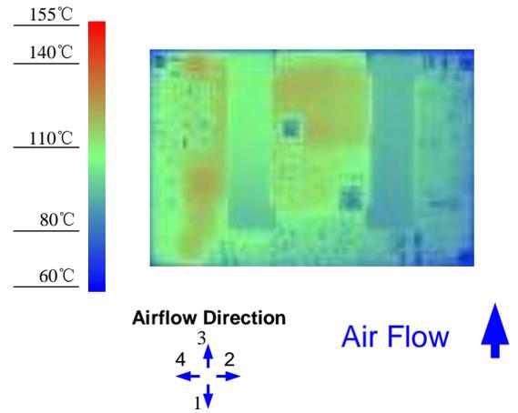
Figure 12. Thermal Image for Airflow Direction 3
