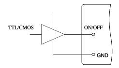
Figure 10. Direct Logic Drive
