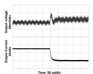
Figure 2. Transient Load Response Input voltage 12V, Output voltage 5V, Output current 3A->0A, Slew rate 1A/µs
