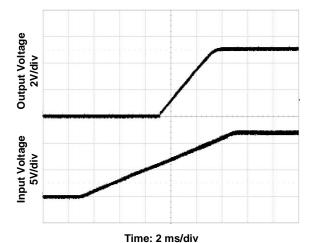
**Figure 7.** Start-Up from Application of Input Voltage Vin = 12V, Vo = 5V, Io = 0A
