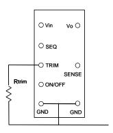
Figure 12. Circuit to Trim Output Voltage.
