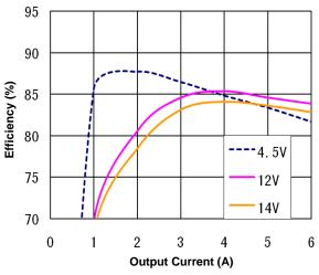
Figure 1(b). Efficiency vs. Load Current (25°C, 1.2V output)
