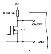
Figure 9. Circuit for Logic Control
