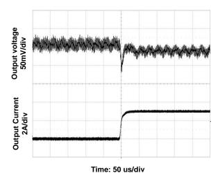
Figure 3. Transient Load Response.
