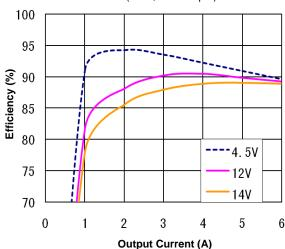
Figure 1(d). Efficiency vs. Load Current (25°C, 2.5V output)
