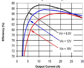
Figure 2a. Efficiency vs. Load Current (25°C)
