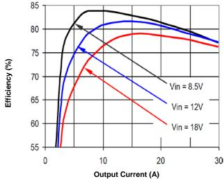
Figure 1a. Efficiency vs. Load Current (25°C)
