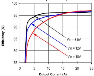
Figure 5a. Efficiency vs. Load Current (25°C)
