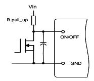
Figure 8. Circuit for Negative Logic Control
