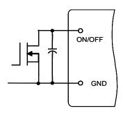
Figure 7. Circuit for Positive Logic Control
