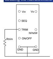
Figure 9. Circuit for Output Voltage Trim
