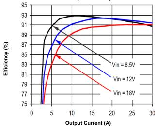
Figure 3a. Efficiency vs. Load Current (25°C)
