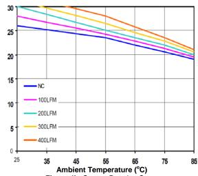
Figure 4b. Current Derating Curve (Vin=12V, open frame)
