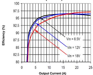
Figure 6a. Efficiency vs. Load Current (25°C)
