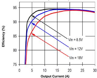
Figure 4a. Efficiency vs. Load Current (25°C)
