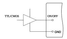
Figure 12. Direct Logic Drive
