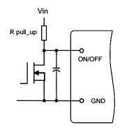
Figure 11. Circuit for Logic Control
