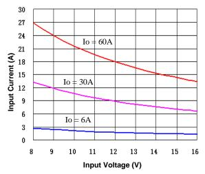
Figure 5.Input Characteristics (3.3V output)
