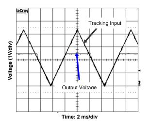
Figure 6.Voltage Tracking/Sequencing (with tracking option) Vin = 12V, Vo = 2.5V, Io = 0A
