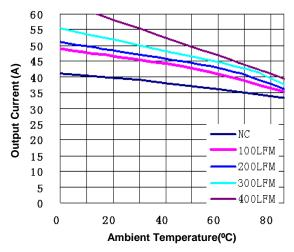
Figure 10(f). CurrentDerating Curve for 2.5V Output
