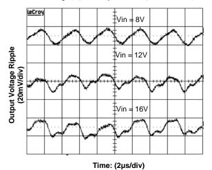
Figure 4.Output Ripple Voltage at 2.5V, 60A Output
