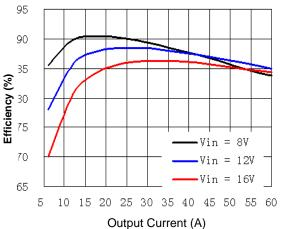
Figure 1(C). Efficiency vs. Load Current (Vout= 1.2V)
