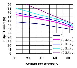
Figure 10(h). Current Derating Curve for 5V Output
