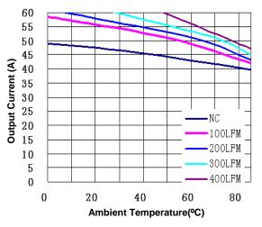
Figure 10(c). Current Derating Curve for 1.2V Output
