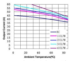
Figure 10(e). Current Derating Curve for 1.8V Output
