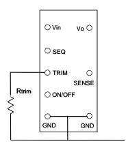
Figure 13. Circuit to Trim Output Voltage.
