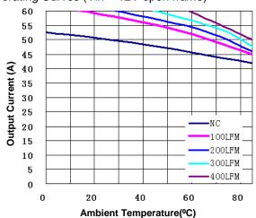
Figure 10(a). Current Derating Curve for 0.8 V Output
