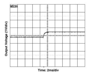
Figure 7.Start-Up with Prebias Input voltage 12V, Output current 0A, Output voltage 2.5V, Prebias 1.8V
