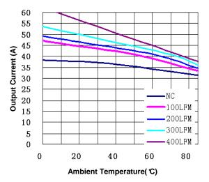
Figure 10(g). Current Derating Curve for 3.3V Output
