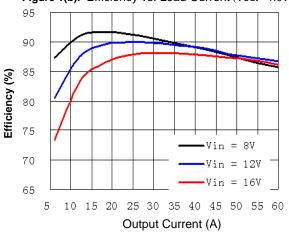
Figure 1(d). Efficiency vs. Load Current (Vout= 1.5V)
