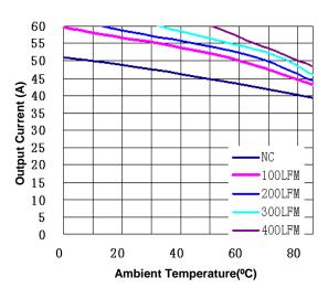
Figure 10(b). Current Derating Curve for 1.0V Output
