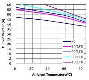
Figure 10(d). Current Derating Curve for 1.5V Output
