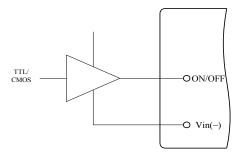
Figure 12. Direct Logic Drive
