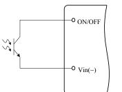
Figure 10. Opto Coupler Enable Circuit
