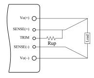
Figure14. Circuit to Increase Output Voltage
