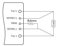
Figure 13. Circuit to Decrease Output Voltage
