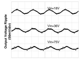
Time – t (2µs /div) Figure 4. Output Ripple Voltage at Full Load
