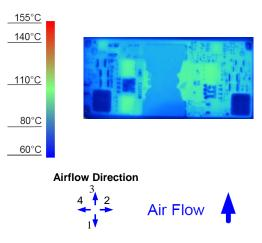
Figure 8. Thermal Image for Airflow Direction 3 (4A output, 55°C ambient, 200 LFM, typical Vin, open frame)
