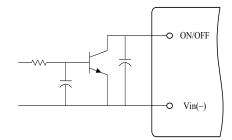
Figure 11. Open Collector Enable Circuit
