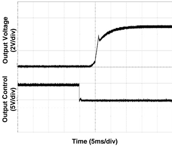
Figure 3. Start-Up from Enable Control
