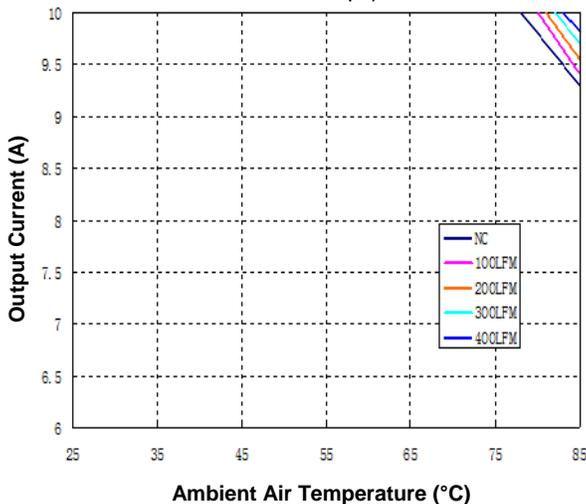
Figure 7. Derating Curve for Airflow Direction 1
