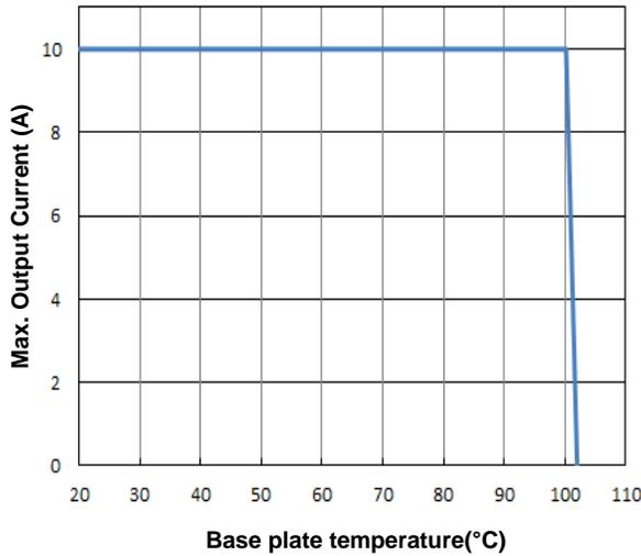
**Figure 9.**Current Derating Curve for Base plate
