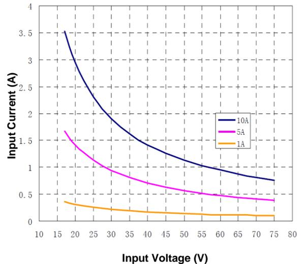
Figure 2. Input Characteristics
