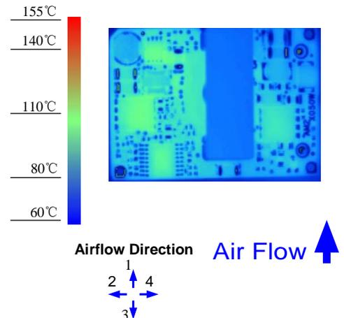
Figure 8. Thermal Image for Airflow Direction 1
