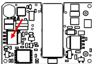
Figure 15. Temperature Monitoring Location
