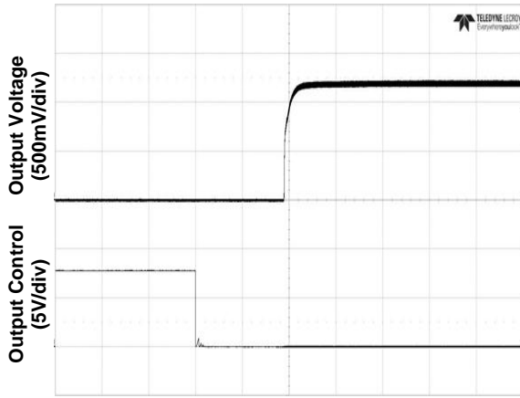
Time - t (5ms/div) Figure 3. Start-Up from Enable Control Input voltage 48V, Output current 100A
