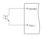
Figure 12.Opto Coupler Enable Circuit
