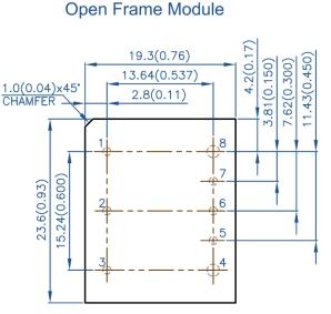
\*Pin 1,2,3,5,6,7 are 1.02 (0.040) dia. \*Pin 4,8 are 1.57 (0.062) dia.
