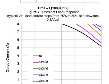
35 45 55 Ambient Temperature (ºC) Figure 9. Current Derating Curve with Open Frame (Direction 3 (Ref. Figure 10); typical Vin, soldered interface)
