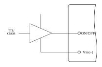
Figure 14. Direct Logic Drive
