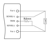
Figure 15. Circuit to Decrease Output Voltage
