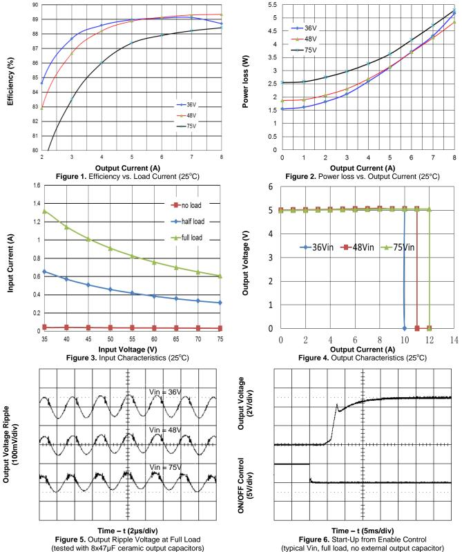
(tested with 8x47µF ceramic output capacitors)
