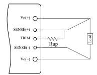
Figure 16.Circuit to Increase Output Voltage
