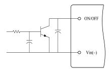
Figure 13. Open Collector Enable Circuit
