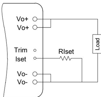
Figure 5. Program Constant Output Current Set Point
