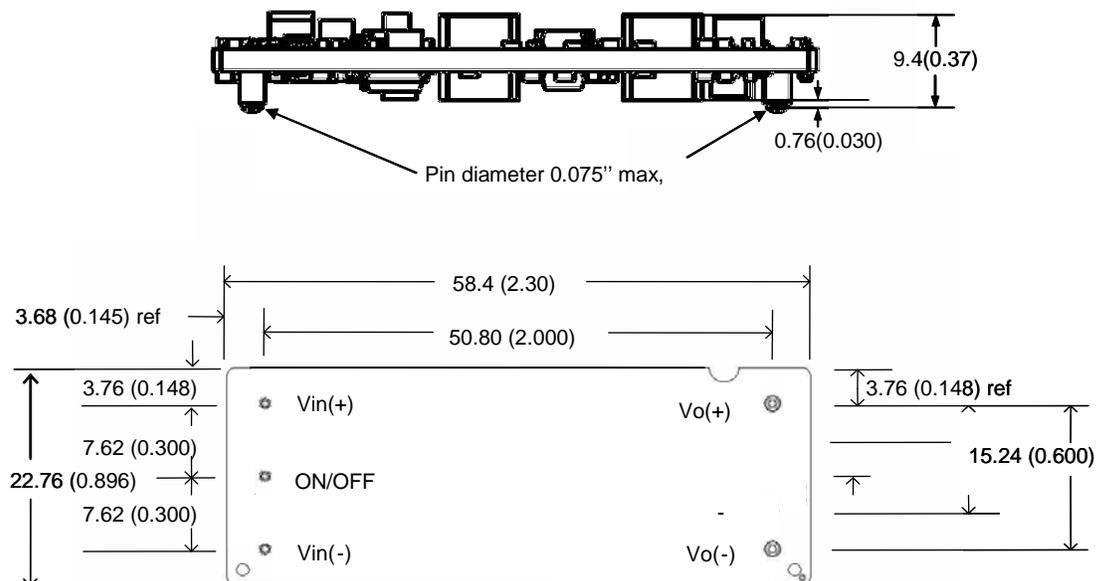
Fig. 1. Mechanical Outline of an SMT Eighth Brick Converter
